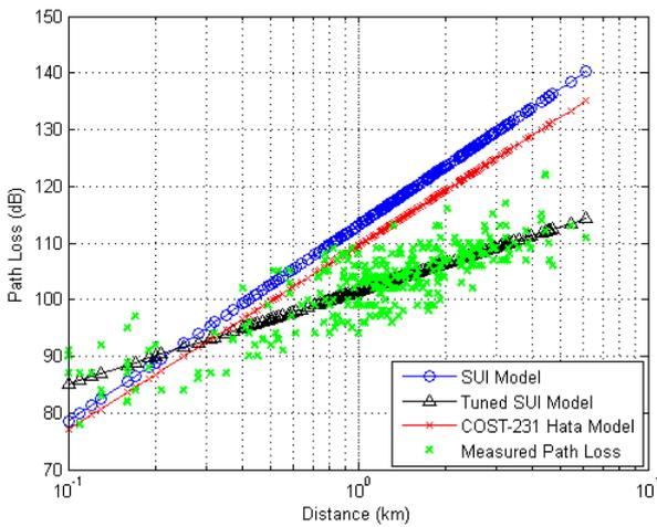
Fig. 3 Tuned propagation models behavior in logarithmic scale
