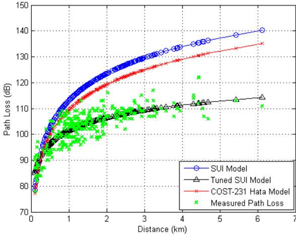
Fig. 2 Propagation models behavior in linear scale
