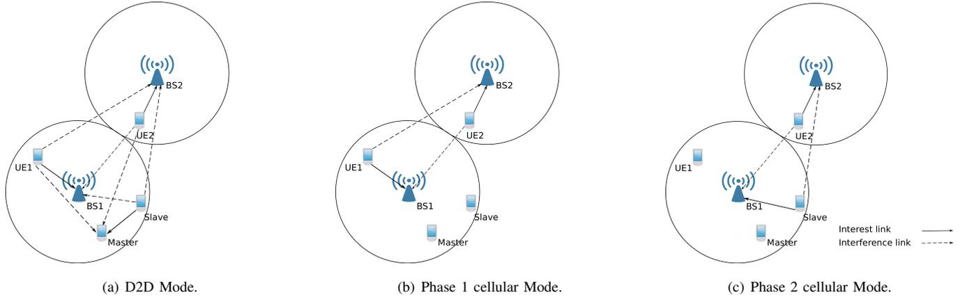
Fig. 1. Study scenario with the interest and interference links for both communication modes: D2D and cellular.
