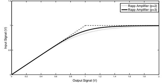
Fig. 1. Transfer Functions of the amplifiers.
