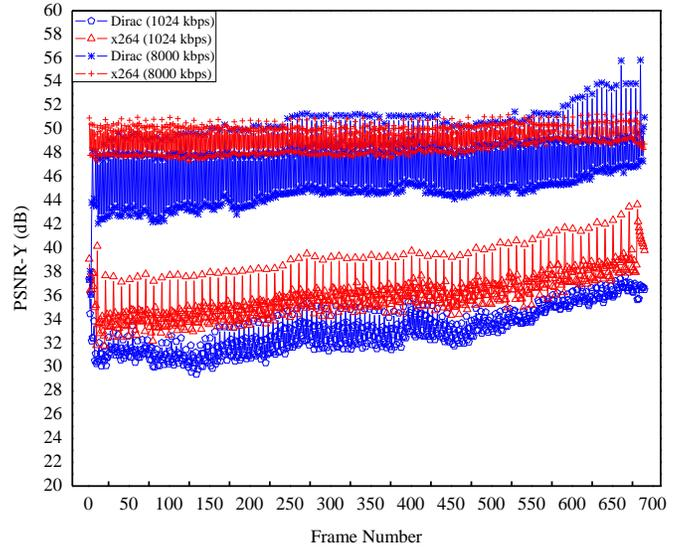
Figure 2. Trend of PSNR (dB) frame by frame with increasing bit rate for the Tractor content at LD resolution.
