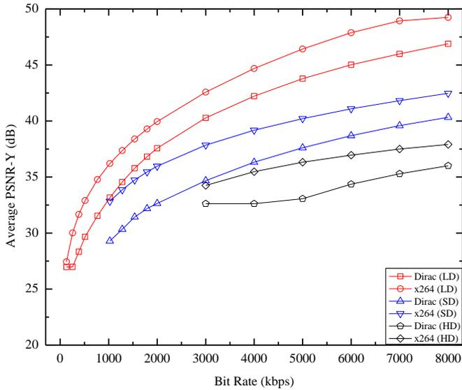
Figure 3. Comparison of average PSNR (dB) of the “Tractor” content after compression at different resolutions (LD, SD and HD).
