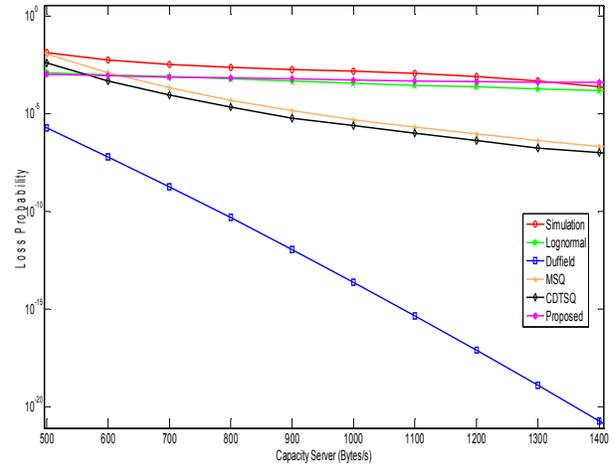
Fig.3. Loss Probability versus Server Capacity for the traffic trace lbl\_pkt\_5
