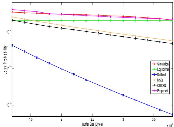
Fig.4. Loss Probability versus Size of Buffer for the traffic trace lbl\_pkt\_5
