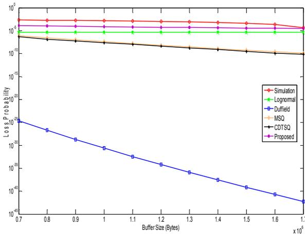
Fig. 6 Loss Probability versus Size of Buffer for the traffic trace dec\_pkt\_1
