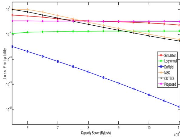
Fig. 5. . Loss Probability versus Server Capacity for the traffic trace dec\_pkt\_1
