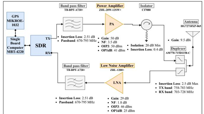
Fig. 1: Adopted radio system structure.
