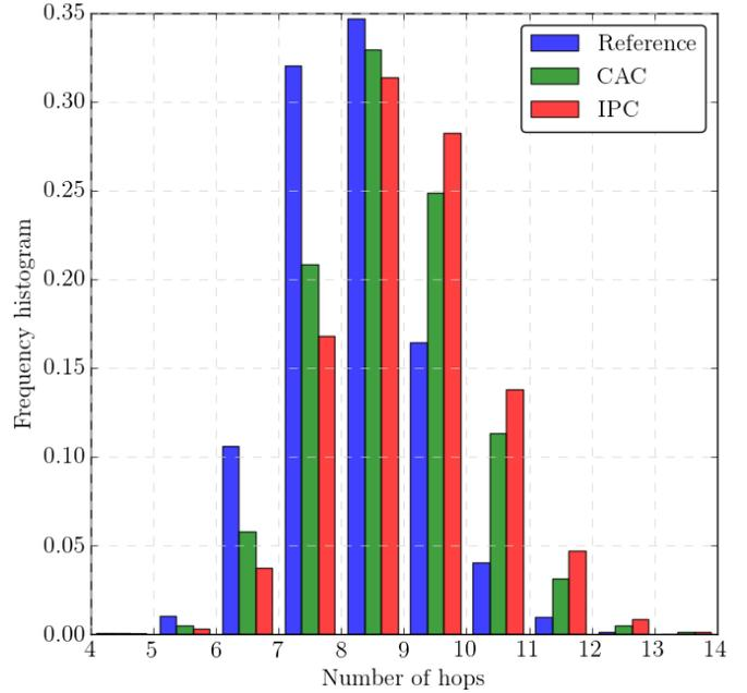
Fig. 5. Frequency histogram of the multihop links between source and sink.
