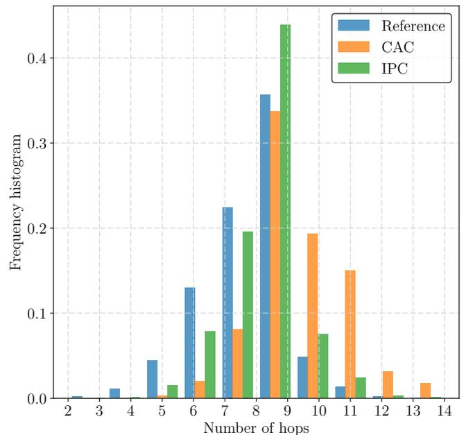
Fig. 6. Frequency histogram of the multihop links between source and sink, considering the SIR experienced by secondary users.
