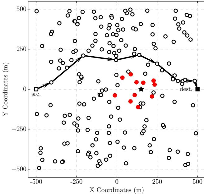
Fig. 2. Multihop link between source and sink nodes in the CAC deployment scenario.
