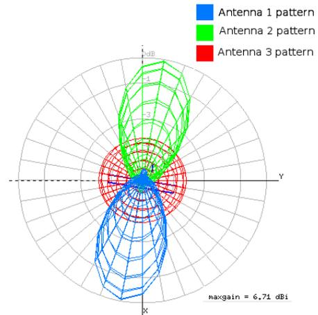
Fig. 5. Resulting antenna pattern for evolved 3x3 MIMO configuration, One cluster. SNR=20dB. Volume= $(0.2\lambda)^3$ .
