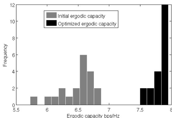
Fig. 4. Histogram for evolved 3x3 MIMO configuration, One cluster. Uniform cluster main direction distribution. SNR=20dB. Volume= $(0.2\lambda)^3$ .
