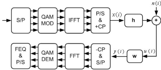
Fig. 1: The diagram of the baseband system model.
