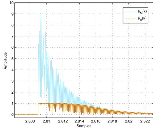
Fig. 3: Behavior of  $e_M(k)$  and  $e_R(k)$  when impulsive noise is added to the output of PLC channel during data communication by using OFDM system discussed in Section II.
