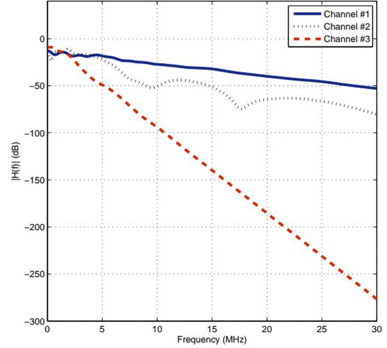
Fig. 2: Spectrum attenuation profile of three PLC channels.
