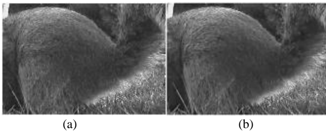
Figure 14. 10 th frame of the squirrel1280 sequence (30% resolution). (a) Dirac-decoded picture with PSNR = 30.3596 and MSSIM = 0,876668. (b) H.264-decoded picture, with PSNR = 33.5563 and MSSIM = 0,929297.
