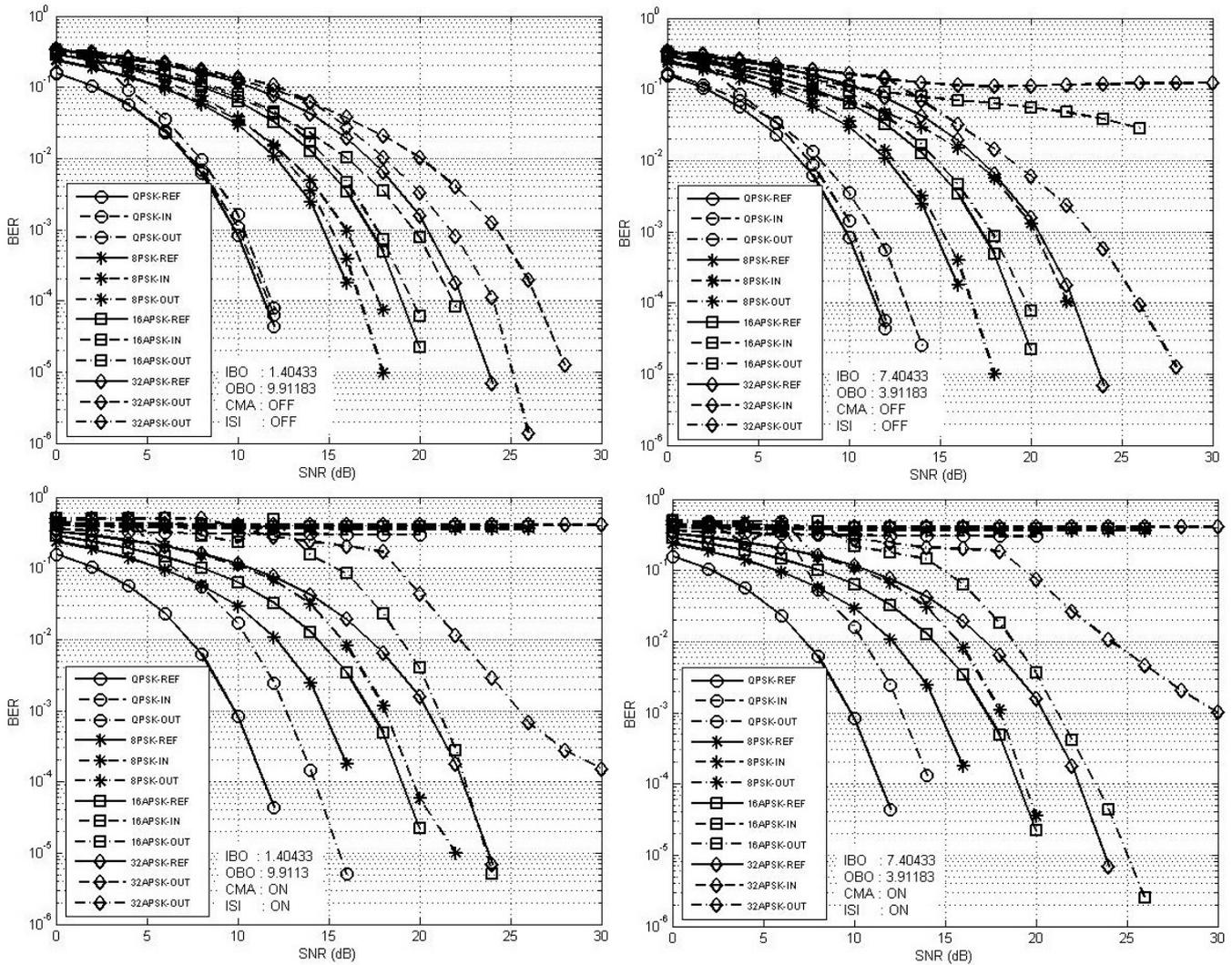
Fig. 4. BER performance for all DVB-S2 modulations (no interleaving and coding), in the presence of severe and moderate nonlinearity (using Saleh model), CMA "on" and "off", with and without ISI. The 6-tap static wireless channel, used in the simulations, was obtained by averaging 100 channel realizations using the Matlab embedded function "rayleighchan". All channel taps present Rayleigh statistics, modeling a complete non-line of sight LMSC.
