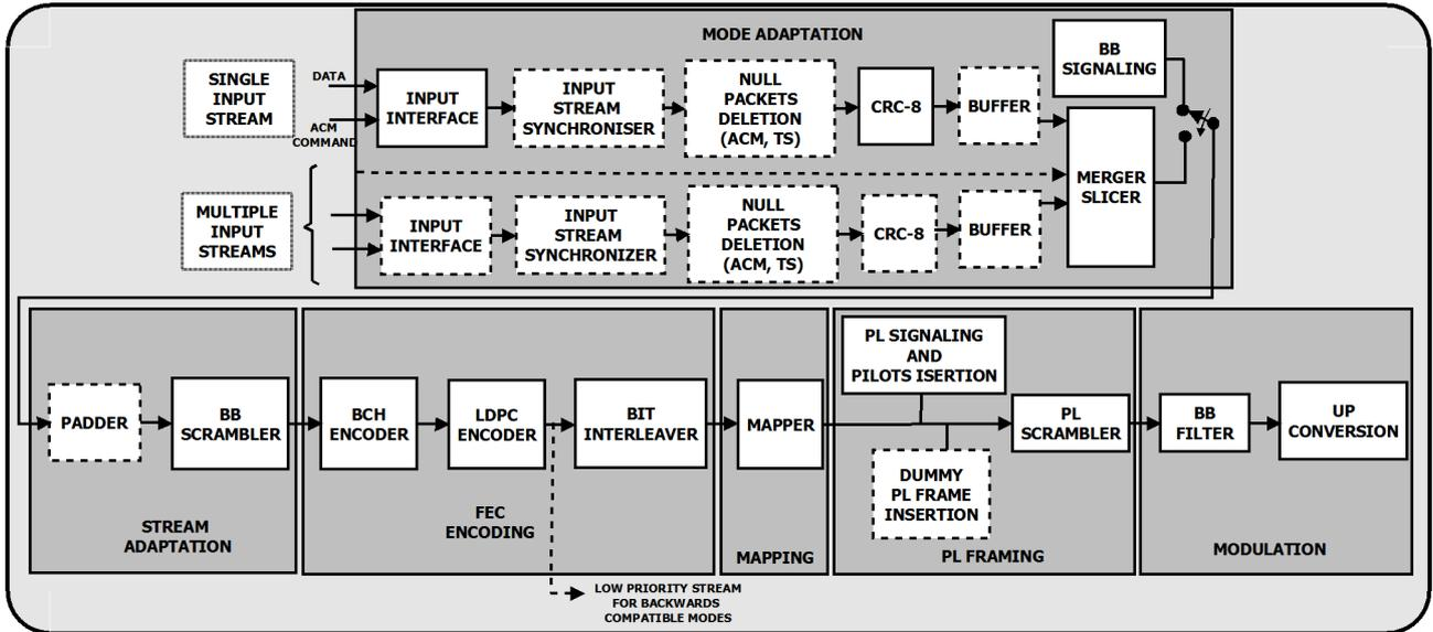
Fig. 1. DVB-S2 transmitter block diagram [6].
