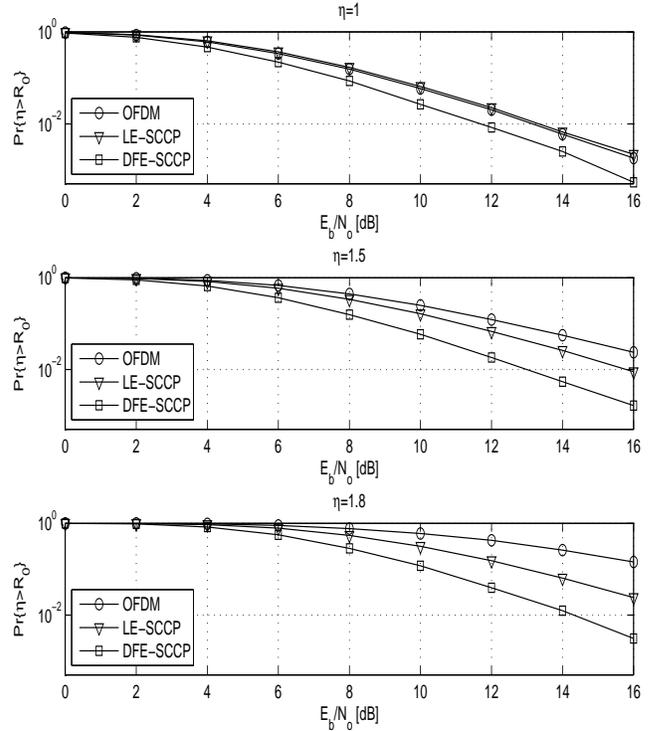
Fig. 2. Cutoff rate outage for QPSK modulation and channel with transfer function given by eq. (38).
