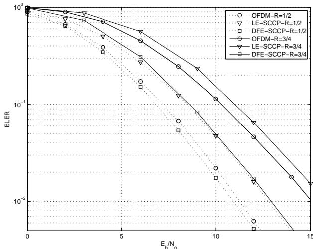
Fig. 3. BLER for QPSK modulation and channel with transfer function given by eq. (38). Error correcting code with generator polynomial  $[133\ 171]_{\text{octal}}$ , coding rates  $R = 1/2$  and  $R = 3/4$
