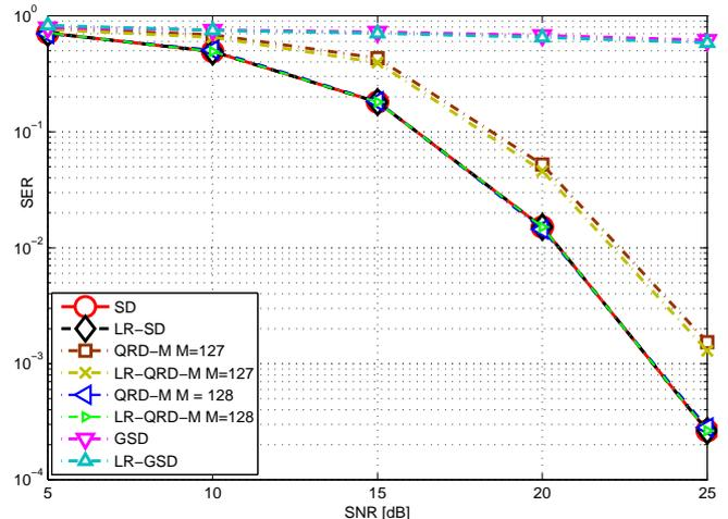
Fig. 4. SER for the SD, QRD-M and GSD detectors in  $m = n = 4$  system and 16-QAM modulation.
