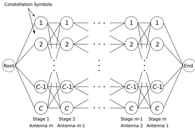
Fig. 3. Flow chart of the GSD for a generic system with  $m$  antennas and modulation with  $C$  symbols.
