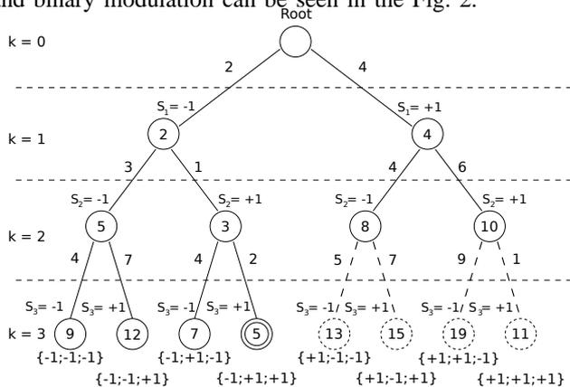
Fig. 2. SD search tree,  $d = 6$ . Numbers at the side of each branch are lengths; numbers inside the nodes are the accumulated metrics; double lined circle indicates the optimal solution; dotted branches are non-visited nodes.
