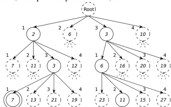
Fig. 1.  $M$  algorithm. The numbers outside the circles are the symbols of the constellation (nodes), those inside the circles are the accumulated metric until that node. The solid circles are the  $M$  nodes chosen by the algorithm in each layer, while the dotted ones are the excluded nodes. Dotted lines indicate the not expanded branches. The double lined circle shows the obtained solution.
