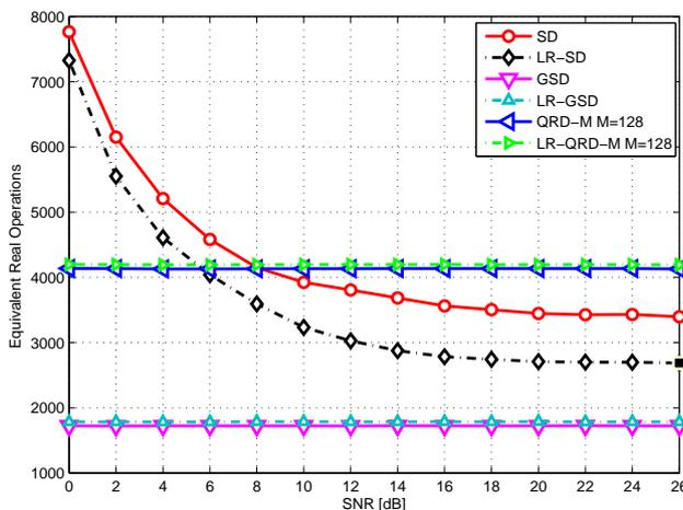
Fig. 5. Equivalent Real Operations obtained from the equivalent computational time versus SNR. System with  $m = n = 4$  and 16-QAM modulation.
