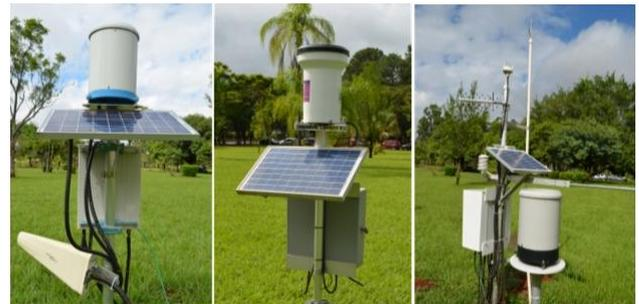
Fig. 1. Pictures showing the most common DCP models installed. From left to right, (a) DCP-Pluvio, (b) DCP-Acqua and (c) DCP-Agro.
