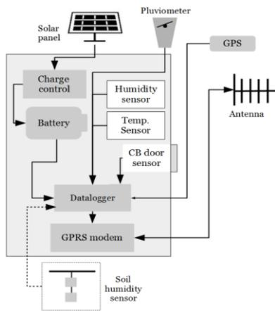
Fig. 5. Schematic representation of DCP-acqua (added soil humidity sensor) and DCP-pluvio.
