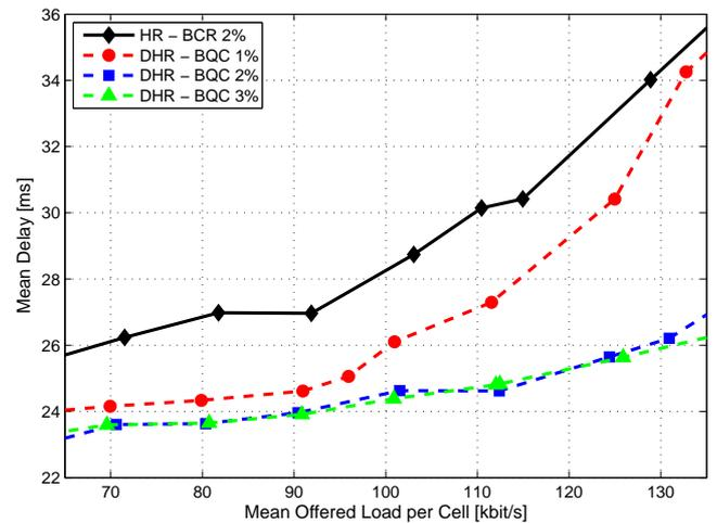
Fig. 4. Mean Net Delay vs Offered Load.
