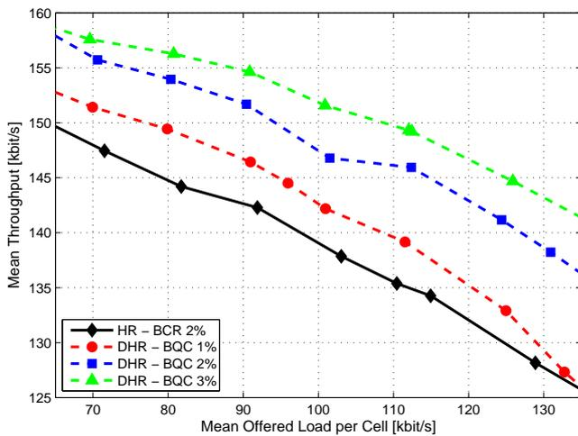
Fig. 2. Mean Net Throughput vs Offered Load.
