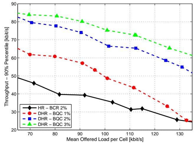
Fig. 3. Net Throughput (90th Percentile) vs Offered Load.
