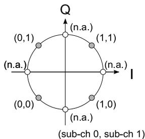
Fig. 1. 8PSK constellation symbols used on OSC.
