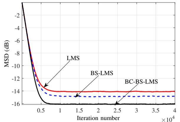
Fig. 4. MSD evolution (in dB) for the LMS, BS-LMS and BC-BS-LMS algorithms.
