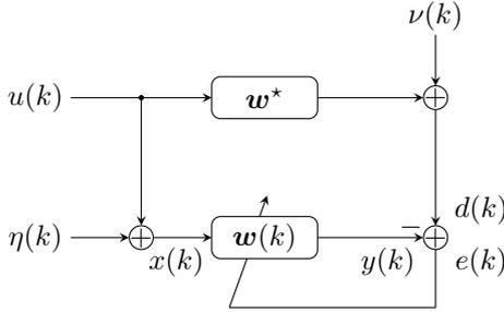
Fig. 2. Block diagram of a system identification adaptive filtering system, where the adaptive filter input is corrupted by noise  $\eta(k)$ .
