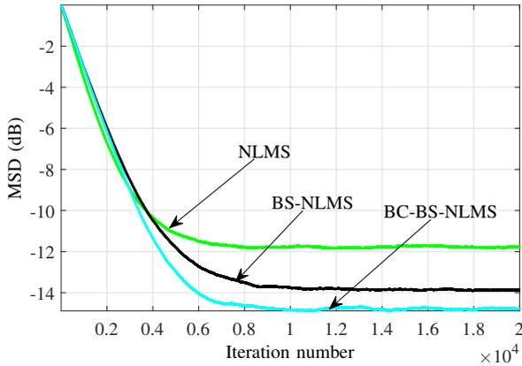
Fig. 5. MSD evolution (in dB) for the NLMS, BS-NLMS and BC-BS-NLMS algorithms.
