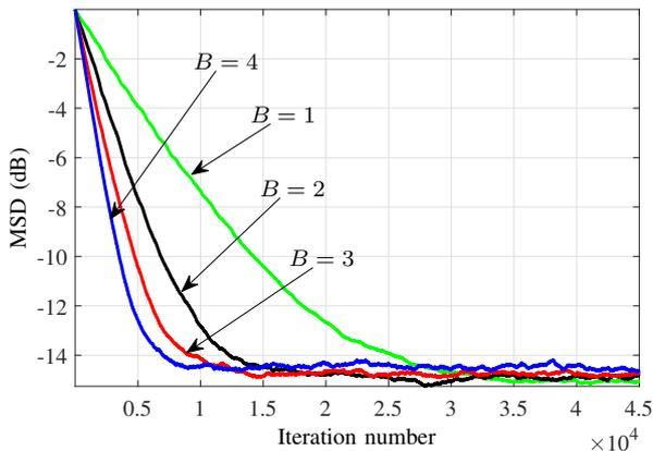
Fig. 6. MSD evolution (in dB) of the SPU-BC-BS-NLMS algorithm for different values of  $B$ .
