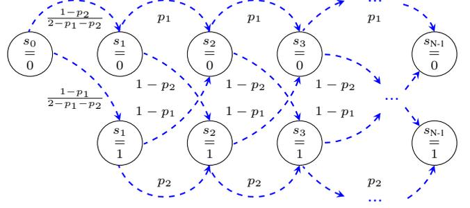
Fig. 3. Diagram for block-sparse model with impulse-response generation.
