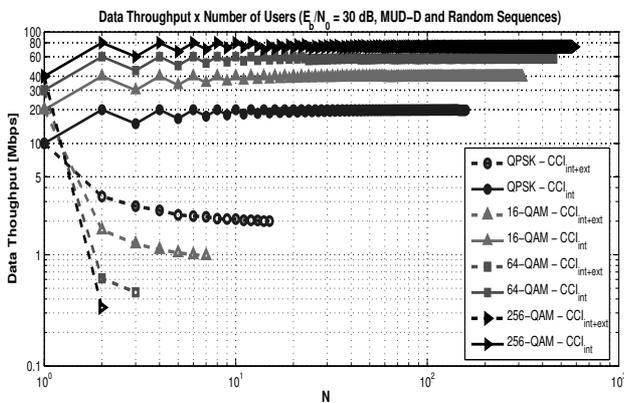
Fig. 5. Data Throughput Versus the Number of Users for a DS-CDMA System with MUD-D Detector and Random Spreading Sequences for  $E_b/N_0 = 30$  dB and QPSK, 16, 64 and 256-QAM Modulations.
