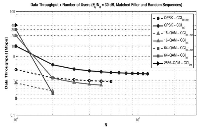
Fig. 3. Data Throughput Versus the Number of Users for a DS-CDMA System with Matched Filter and Random Spreading Sequences for  $E_b/N_0 = 30$  dB and QPSK, 16, 64 and 256-QAM Modulations.
