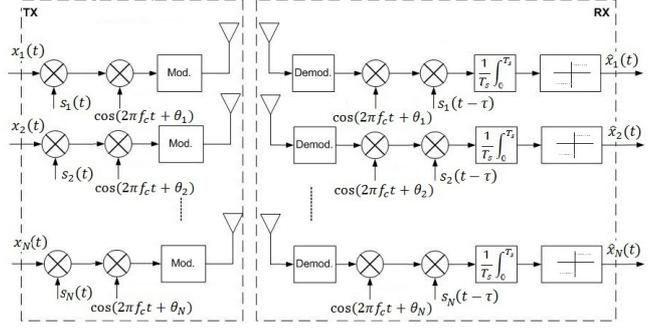
Fig. 1. DS-CDMA Scheme with Matched Filter for  $M$ -ASK Modulation.
