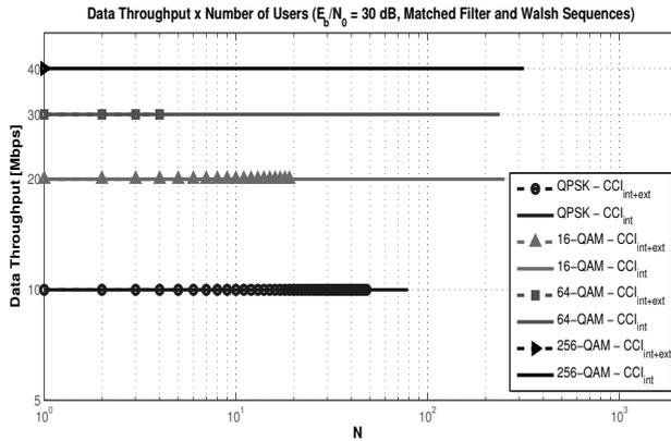
Fig. 4. Data Throughput Versus the Number of Users for a DS-CDMA System with Matched Filter and Walsh Spreading Sequences for  $E_b/N_0 = 30$  dB and QPSK, 16, 64 and 256-QAM Modulations.
