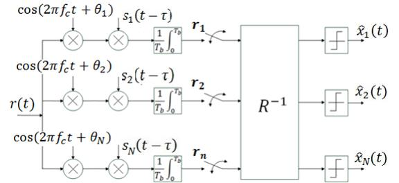
Fig. 2. Scheme of the DS-CDMA Receiver with MUD-D for  $M$ -ASK Modulations.
