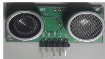
Fig. 3 Sensor de ultrassom TRF05/SRF05
