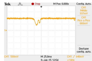
Fig. 1 – Waveform presented by a passing drop through the sensors.
