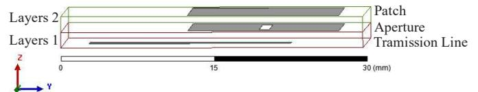
Fig. 1. Structure of aperture-coupled antenna.
