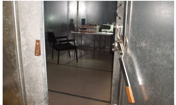
Fig. 3 – Measurement setup inside the EMI shielded room.
