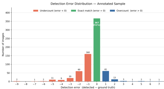
Fig. 3: Signed detection error distribution (detected – ground truth) across the annotated subset; under-detection is the dominant failure mode.
