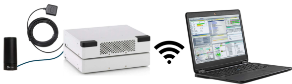
Fig. 1: Measurement setup: a GPS antenna, a TSM-6B mobile network scanner, a receiver antenna, and a laptop.
