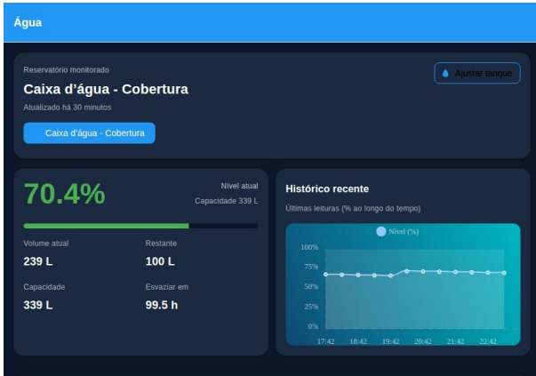
Figure 2. Web dashboard: real-time reservoir status, consumption trends, and alert management.
