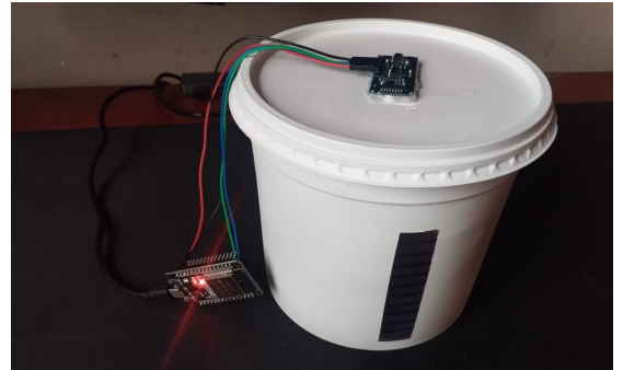
Figure 3. Laboratory prototype: ESP32, HC-SR04, and 1.0 L reservoir.
