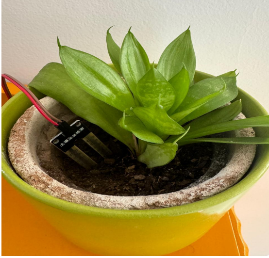
Fig. 1. Prototype of the automated irrigation system with a soil moisture sensor, ESP32, and condensation water for irrigation.
