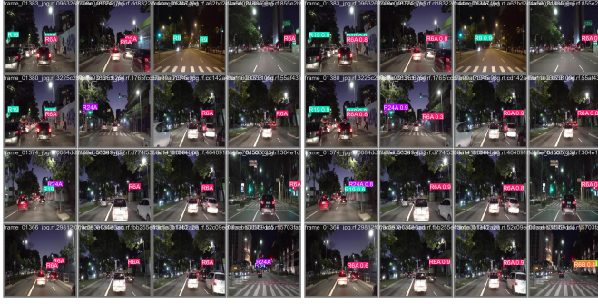
Figure 2. Example of labeled (left) and predicted (right) traffic signs.
