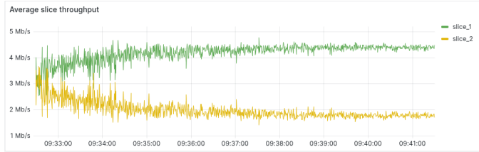
Fig. 5: Average throughput over time for two network slices, with slice 1 maintaining higher rates than slice 2.
