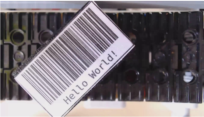
Fig. 13. Frame not detected by YOLO but successfully read by Method 2.
