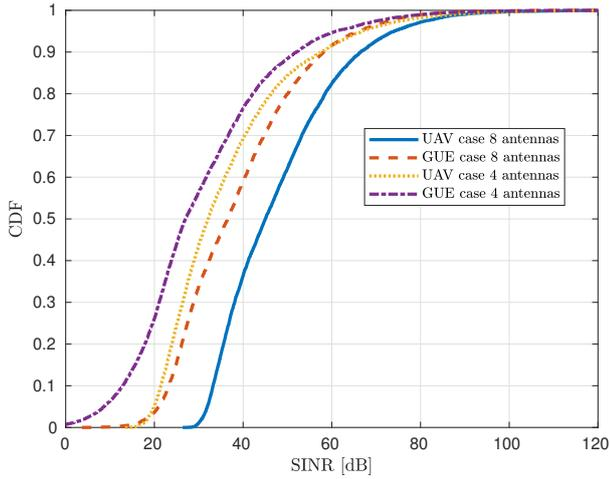
Fig. 2: CDF of SINR: beam towards the UAV.
