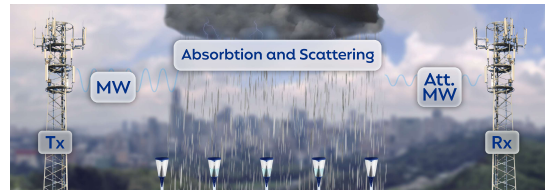
Fig. 1: Illustration of the basic operating principle of CML rainfall estimation.
