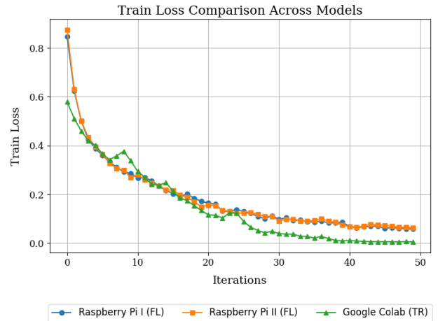
Fig. 2. Comparing the training loss presented by the SqueezeNet model in traditional and federated approach.
