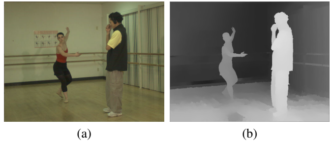
Fig. 1. (a) The Ballet sequence (size 1024x768), view 2, frame 0 and (b) a corresponding gray scale depth map.
