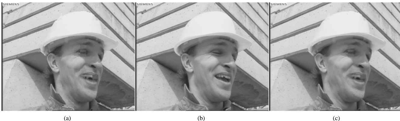
Fig. 3. (a) Regular block motion compensation. (b) Original frame. (c) Overlapped block motion compensation.
