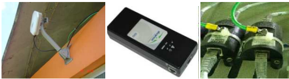
Figure 4. SU components: panel directional antenna and ODU, IDU, and the peak suppressor.
