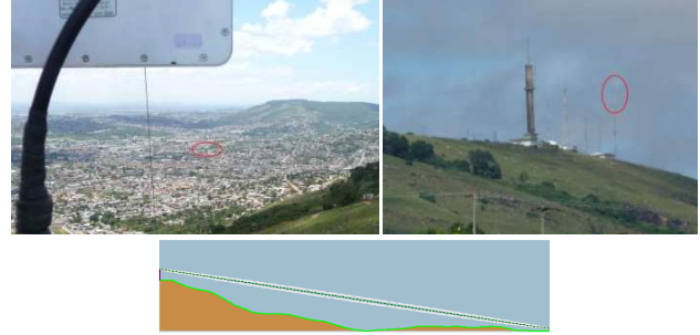
Figure 3. (a) View from AU antenna located at Police Hill. It is also shown the approximate location of the CPE. (b) Location of AU antenna in Police Hill; (c) Fresnel zone visualized using the Radio Mobile software.
