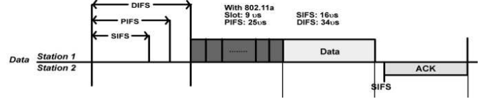
Figure 7. Atomic basic positive acknowledgment (ACK) of data.
