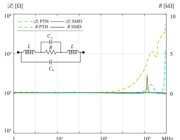
Fig. 1: The impedance magnitude and the resistance value  $R$  of PTH and SMD resistors for the 100  $\Omega$  value.
