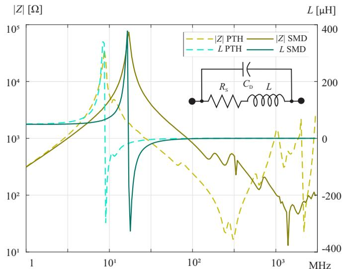
Fig. 3: The impedance magnitude and the inductance value  $L$  of PTH and SMD inductors for the  $47 \mu\text{H}$  value.
