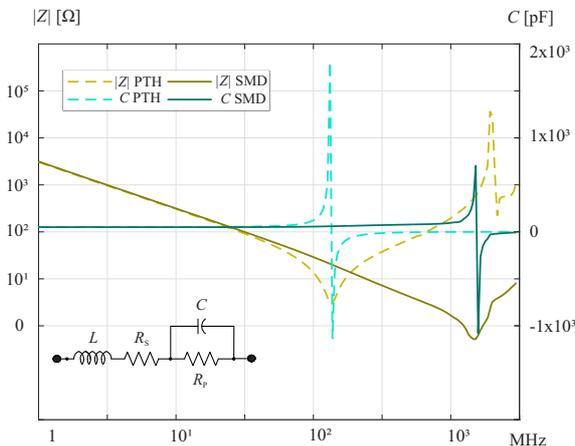
Fig. 2: The impedance magnitude and the capacitance value  $C$  of PTH and SMD capacitors for the  $56 \text{ pF}$  value.
