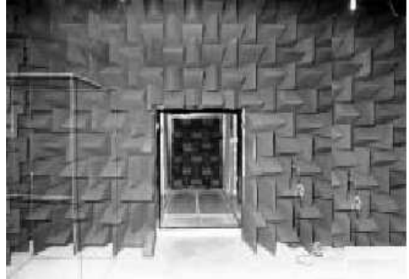
Fig. 2. Semi-anechoic room used for recordings.
