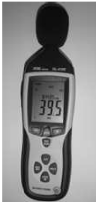
Fig. 4. Digital sound level meter used to adjust the noise volume.
