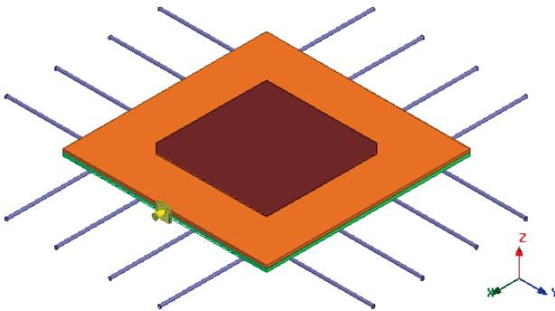
Fig. 7. Structure of the designed antenna with cylindrical rods.
