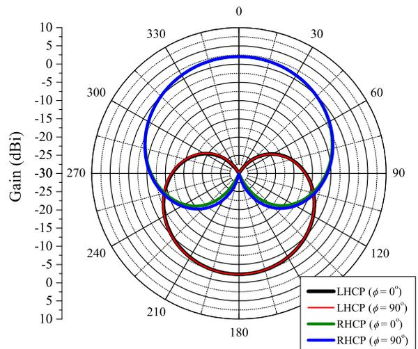
Fig. 6. Gain pattern for the single antenna.
