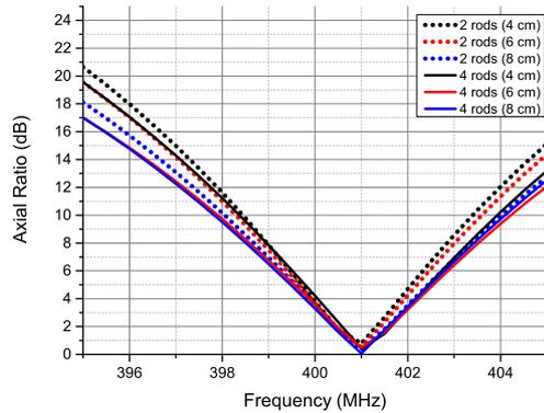
Fig. 14. Axial ratio as a function of the frequency for all cases of the rectangular rods.
