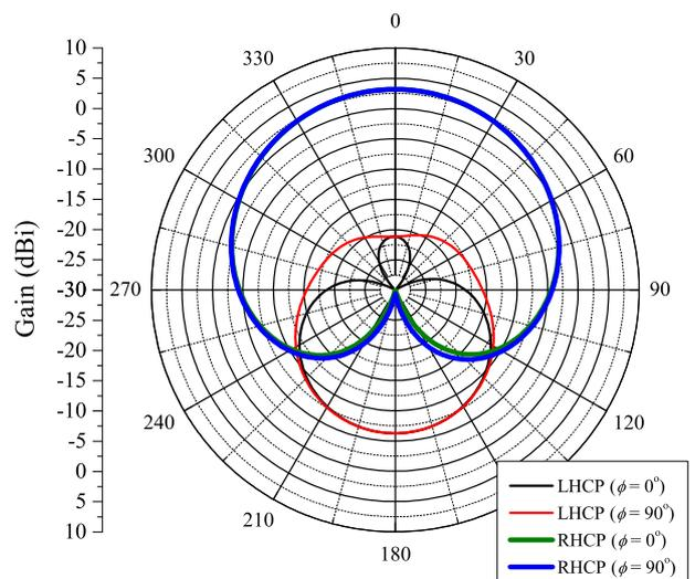
Fig. 10. Gain patterns for the antenna with two 8-cm cylindrical rods attached to each GND edge.
