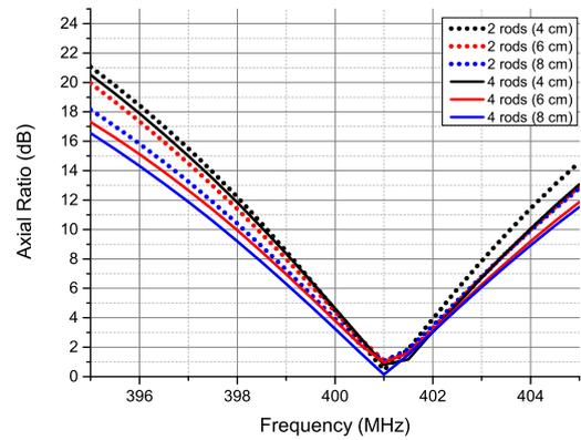
Fig. 9. Axial ratio as a function of the frequency for all cases employing cylindrical rods.
