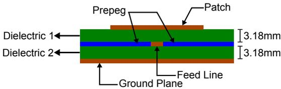
Fig. 2. Cross-sectional view of the designed antenna.
