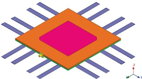
Fig. 12. Structure of the designed antenna with rectangular rods.
