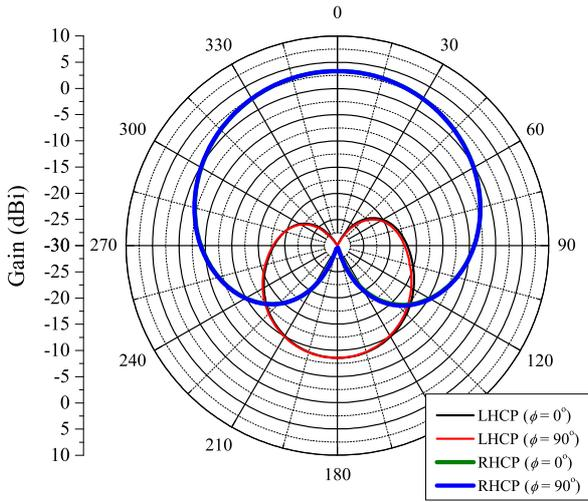
Fig. 11. Gain patterns for the antenna with four 8-cm cylindrical rods attached to each GND edge.
