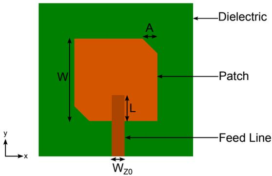
Fig. 3. Top view of the designed antenna.
