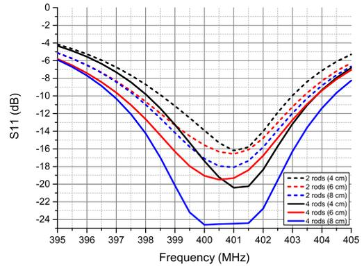
Fig. 8. Reflection coefficient as a function of the frequency for all cases employing cylindrical rods.
