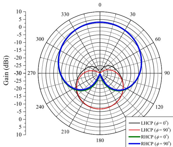
Fig. 15. Gain for the antenna with two rectangular rods and length of 8 cm.
