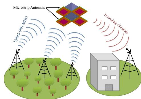
Fig. 1. Scenario for the meteorological nano-satellite.
