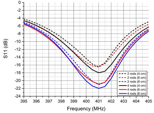
Fig. 13. Reflection coefficient as a function of the frequency for all cases of the rectangular rods.
