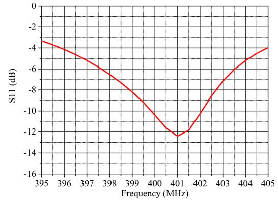
Fig. 5. Reflection coefficient as a function of the frequency for the single antenna.
