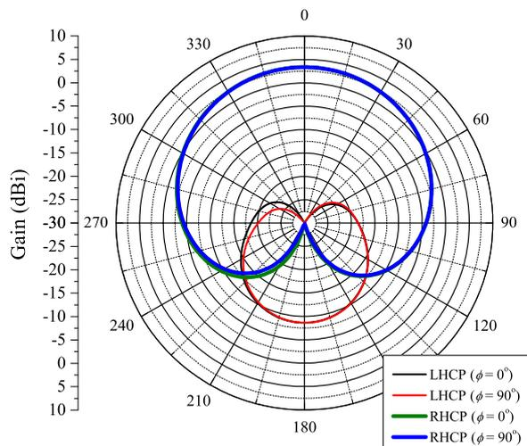
Fig. 16. Gain for the antenna with four rectangular rods and length of 8 cm.
