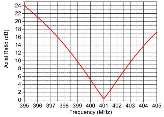
Fig. 4. Axial ratio as a function of the frequency for the single antenna, in  $\theta = \phi = 0^\circ$ .
