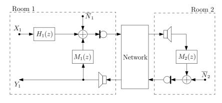
Fig. 4. Simplified teleconference model. Only the transmission/reception cycle for talker 1 is considered.
