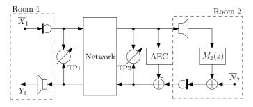
Fig. 6. Feedback path model. TP in the diagram stands for "test point"
