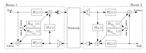
Fig. 1. Complete teleconference model. Figure adapted from [2].
