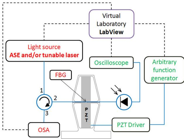
Fig. 3. Experimental setup for measuring the tuning speed.
