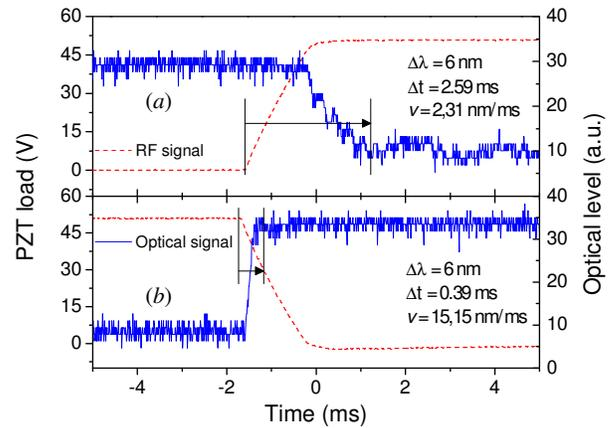
Fig. 4. (a) Rise of the PZT load and (b) drop of the load. For the case when the load increases, the PZT experiences a blocking force.
