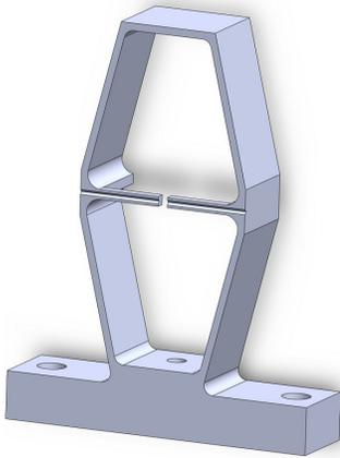
Fig. 1. Metal frame used in the compression-based device.
