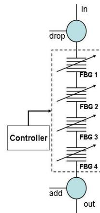
Fig 5. Configuration of the proposed reconfigurable OADM.
