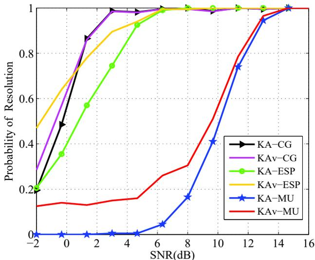
Fig. 1. Probability of resolution of the KA versions and KAv versions of CG, ESPRIT and MUSIC versus SNR with  $M = 12$ ,  $N = 180$ ,  $P = 2$ ,  $L = 200$  runs, unknown uncorrelated sources at  $(89.05, 90.95)^\circ$
