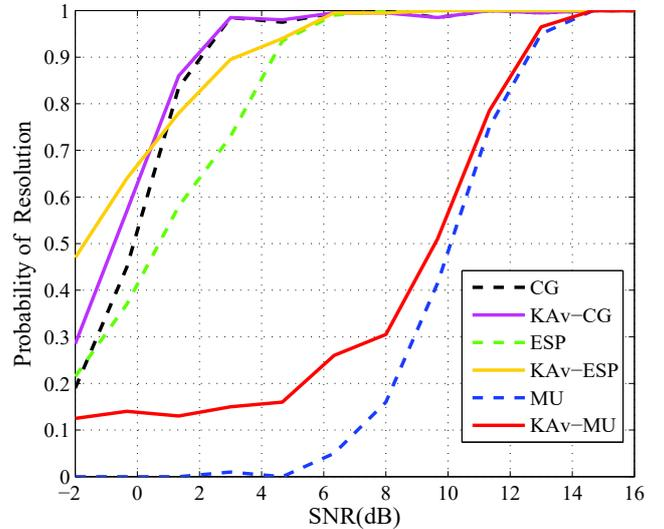
Fig. 2. Probability of resolution of the KA versions and original versions of CG, ESPRIT and MUSIC versus SNR with  $M = 12$ ,  $N = 180$ ,  $P = 2$ ,  $L = 200$  runs, unknown uncorrelated sources at  $(89.05, 90.95)^\circ$
