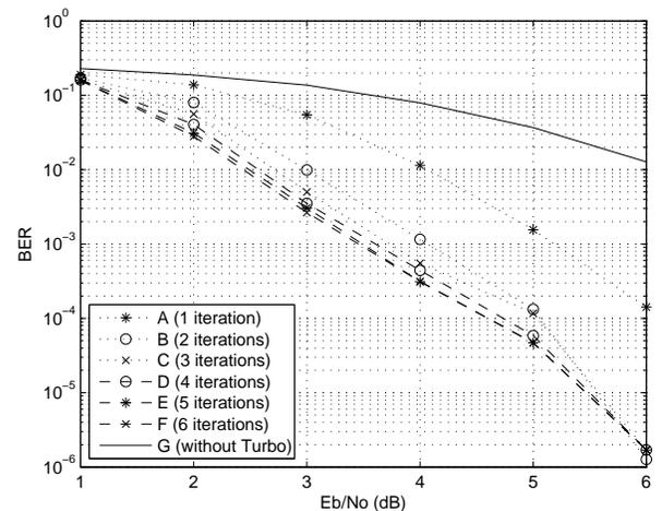
Fig. 6. Bit error rate for user 1, for a rate 1/3 turbo convolutional code with polynomial generator matrix  $\begin{bmatrix} 1 & (1+D^2) \\ 1 & (1+D+D^2) \end{bmatrix}$ .
