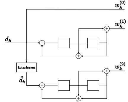
Fig. 3. Encoder for code  $C_2$ , employing two identical polynomial generator matrices, namely  $\begin{bmatrix} 1 & D+D^2 \\ 1+D+D^2 & \end{bmatrix}$ .
