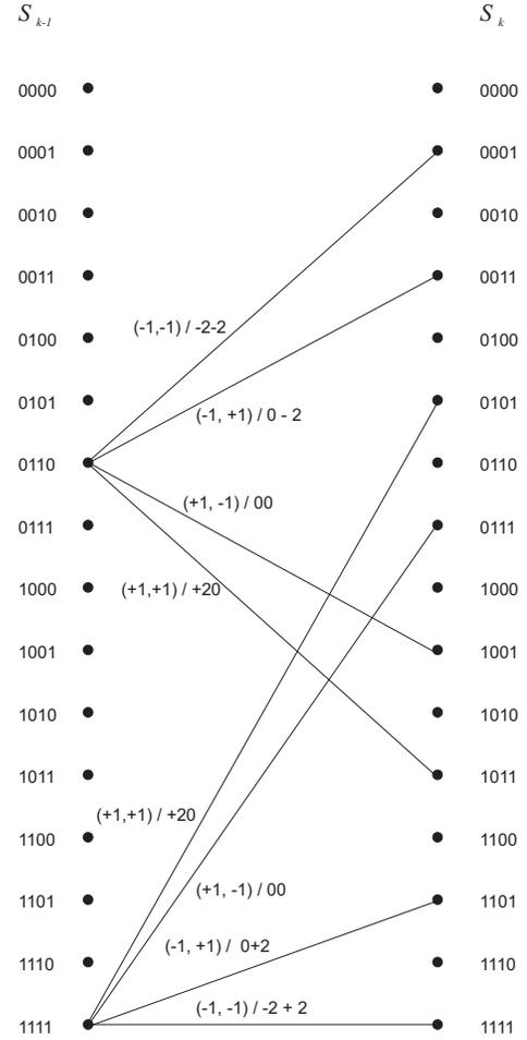
Fig. 4. Branches of the 2-user trellis connecting states  $S_{k-1} = 0110$  and  $S_{k-1} = 1111$ , at time instant  $t = k-1$ , to the corresponding states  $S_k$  at time instant  $t = k$ . For example, if  $S_{k-1} = 0110$  and  $S_k = 0011$ , then  $(u_k, d_k)/\mathbf{x}_k = (-1, +1)/0-2$ .
