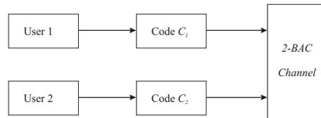
Fig. 1. Model of coding scheme for the 2-BAC.
