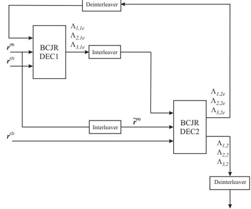
Fig. 5. Iterative decoder, containing two component decoders connected in series.
