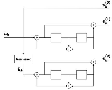
Fig. 2. Encoder for code  $C_1$ , employing two identical polynomial generator matrices, namely  $\begin{bmatrix} 1 & 1+D^2 \\ 1+D+D^2 & \end{bmatrix}$ .
