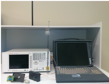
Fig. 2: Spectrum sensing setup using the antenna and the power line cable.
