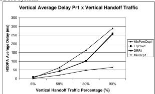
Fig. 2. HSDPA Average Packet Delay Priority 1 in Function of Vertical Handoff Traffic
