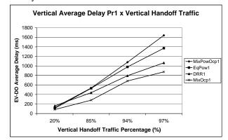
Fig. 3. 1xEV-DO RA Average Packet Delay Priority 1 in Function of Vertical Handoff Traffic
