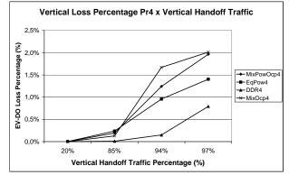
Fig. 6. 1xEV-DO RA Loss Percentage Priority 4 in Function of Vertical Handoff Traffic
