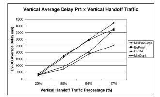
Fig. 4. 1xEV-DO RA Average Packet Delay Priority 4 in Function of Vertical Handoff Traffic
