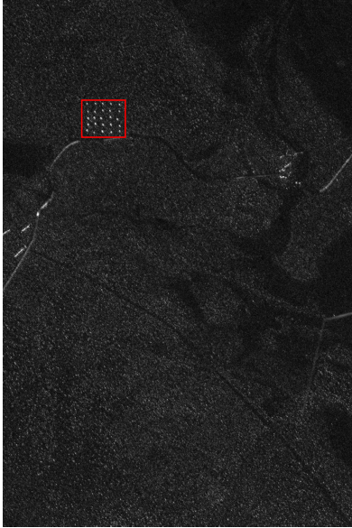
Fig. 1. Example of a SAR image from the CARABAS-II database. The targets are highlighted inside the red square.
