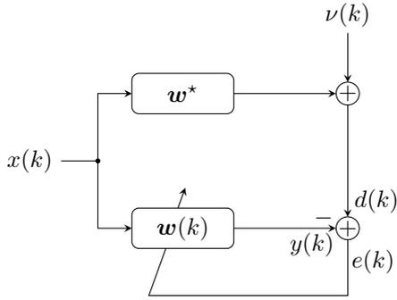
Fig. 1. Block diagram of an adaptive system identification task, where  $\mathbf{w}^*$  denotes the unknown system.
