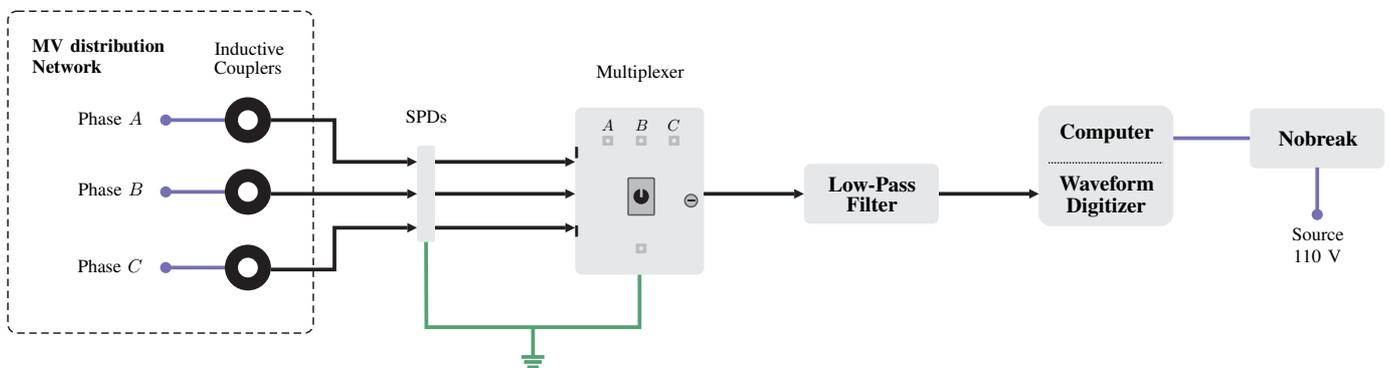
Fig. 2. Block diagram of the sounding-based measurement setup, RX.
