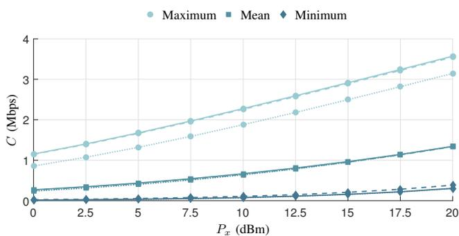
Fig. 5. Achievable data rate versus total transmission power for phases A(-), B(-), and C(:).
