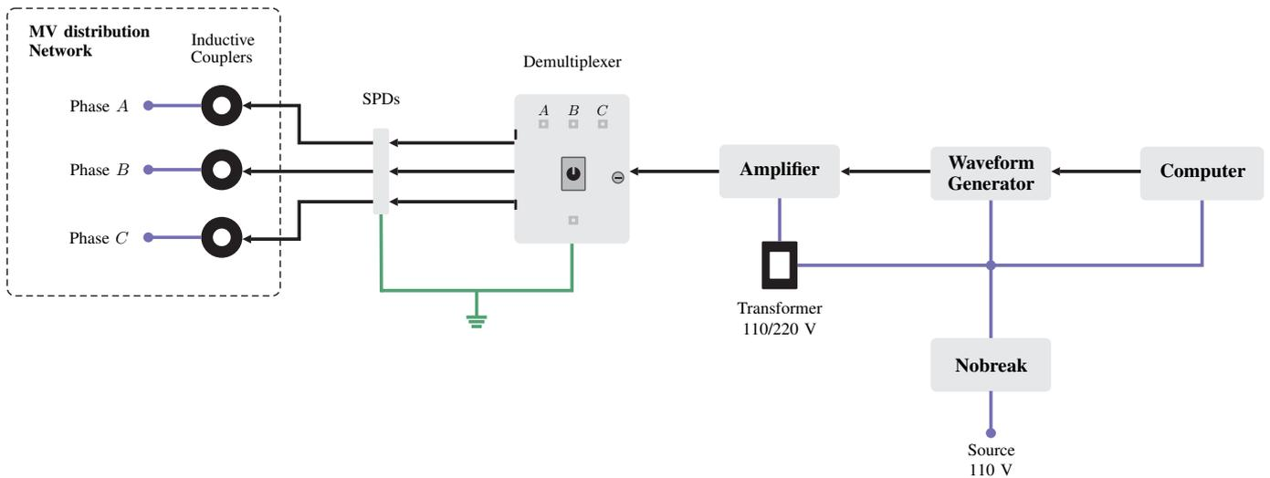
Fig. 1. Block diagram of the sounding-based measurement setup, TX.
