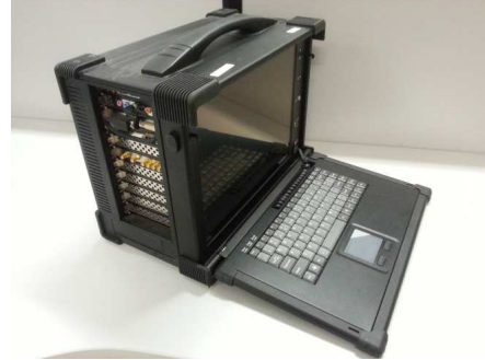
Fig. 3. Rugged computer with the data acquisition board.
