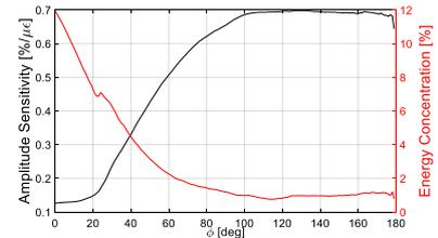
Fig. 4. Amplitude sensitivity and energy concentration as a function of  $\phi$ .
