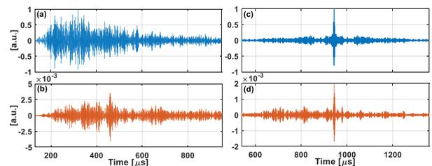
Fig. 1. Original reference signal (a), new reference signal with filtering technique at  $\phi = 30^\circ$  (b), original time-reversal signal (c) and new time-reversal with filtering technique at  $\phi = 30^\circ$  (d)
