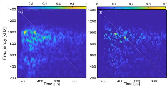
Fig. 2. Absolute value of the STFT of the original (a) and (b) filtered with at  $\phi = 30^\circ$  reference signals. The color bar indicates the coefficients' intensity.
