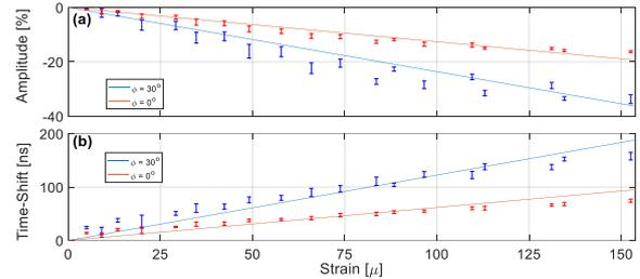
Fig. 3. Peak reduction (top) and time-shift (bottom) as a function of the strain. Symbols are experimental points, lines are linear fit. Blue bars and curves indicate reference signal obtained with  $\phi = 30^\circ$  and red bars and curves indicate measurements without filtering.
