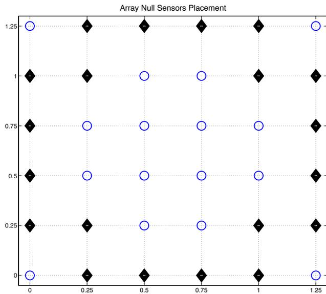
Fig. 7. 2D Constrained Array Null Sensors (O) Placement.
