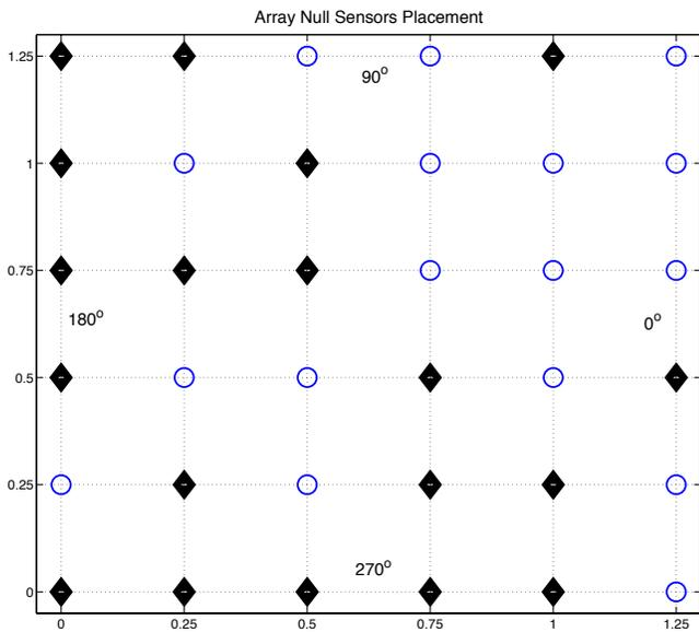
Fig. 4. 2D Constrained Array Null Sensors (O) Placement.
