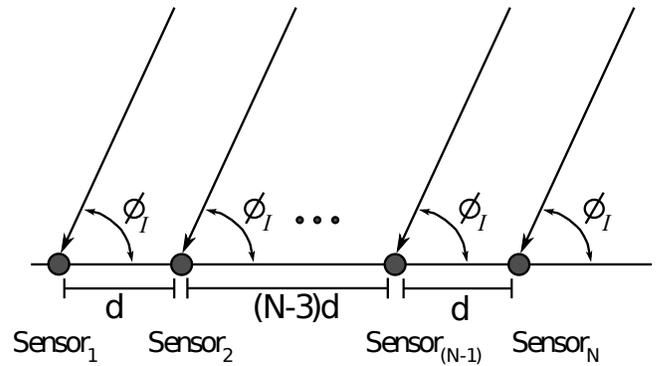
Fig. 2. The Geometry of a Uniform Linear Array (ULA) of sensors.
