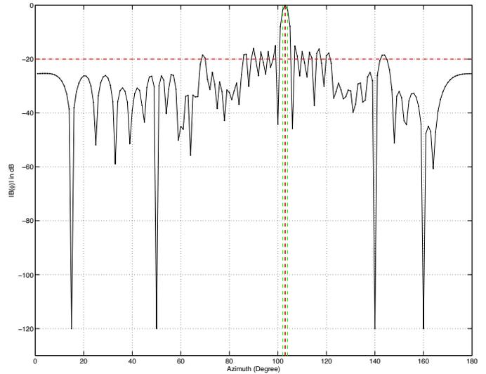
Fig. 5. Constrained Uniform Linear Array Synthesis using SOCP.
