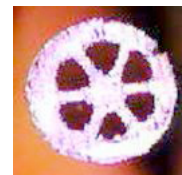
Fig. 1. Micro-photo of the PMMA QD-doped star-6 type mPOF.
